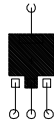
b. 95^\circ\text{C}/\text{W} when mounted on a 0.066\text{ in}^2 pad of 2oz Cu.
