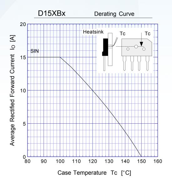
Sine wave R-load with heatsink
